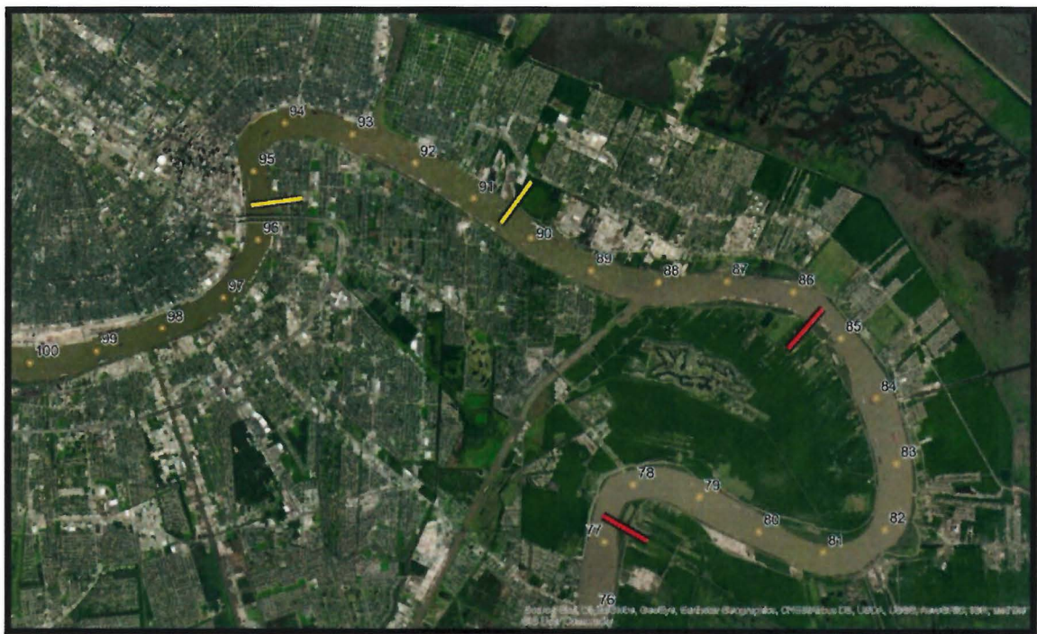
Figure 5. Crossover Points on the Mississippi River Levee: Existing (red) and With-Project (yellow)
